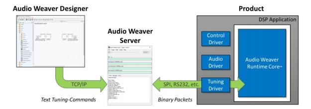
The text-based commands may also be generated by external tools and scripts rather than by Designer. An example script, written in python, that connects to the AWE Server at port 15001 and reads and writes a module's variable in an active layout in real-time is shown below.
